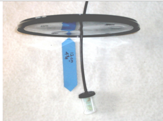
Tube and filter fitted to lid
